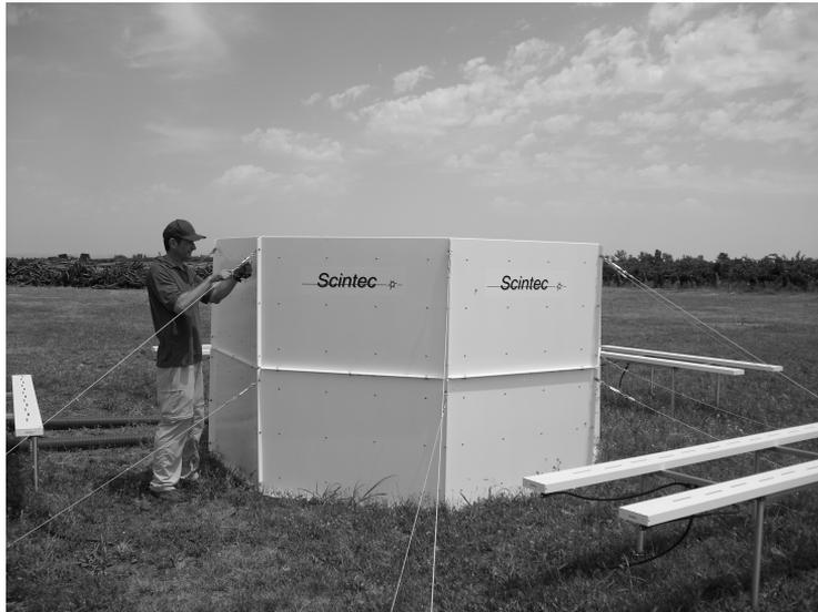
**Figure 7.5:** The WindRASS installed in Raimat since July 1st, 2009.
